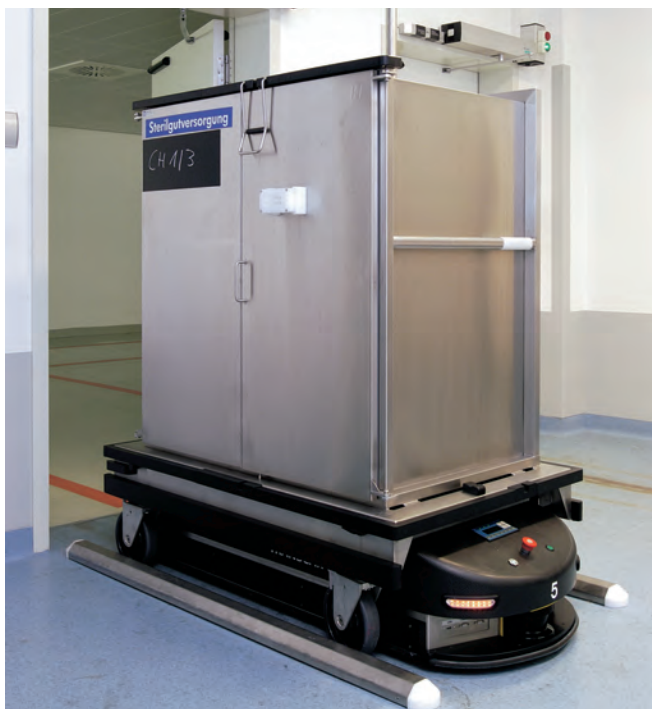
AGV transport cart is collected automatically
