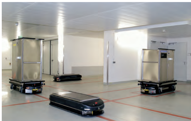
AGV transport units are routed automatically to their destination
